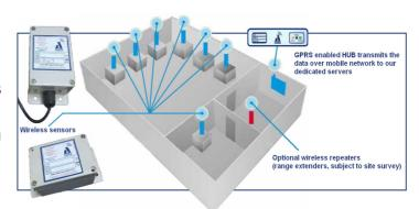
Sensors are installed in the areas to be monitored. The base station sends the data back to our servers. The information is presented to customers, via a website, to manage and view their records and alarms.
